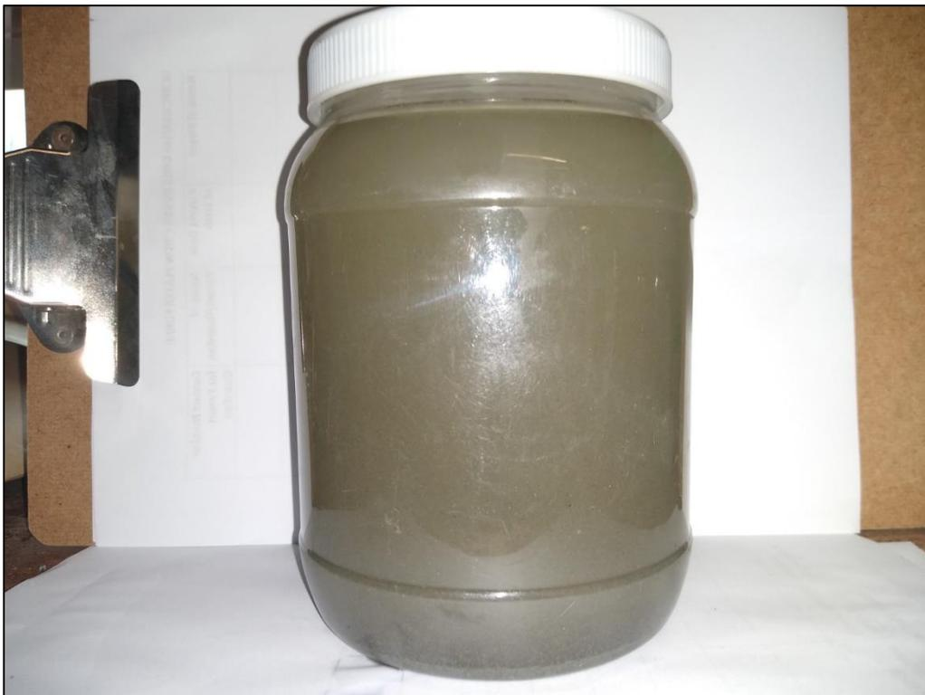
**Photograph 2: Effluent after 1 hour settlement time**
